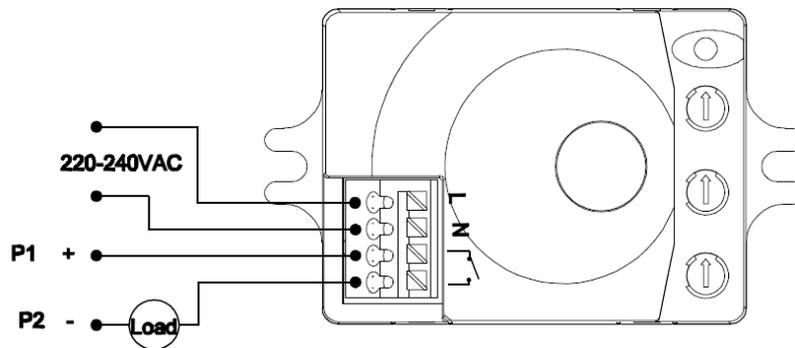
This product is using microwave motion detection function to give dry closing contact signal for the controlled system (this signal is passive dry closing contact signal only.)
