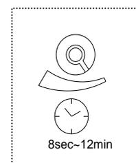
The light can be set to stay ON for any period of time between approx. 8sec (turn fully anti-clockwise) and a maximum of 12min (turn fully clockwise). Any movement detected before this time elapse will re-start the timer. It is recommended to select the shortest time for adjusting the detection zone and for performing the walk test.
