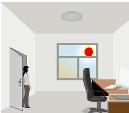
With ambient light more than daylight threshold, the lamp does not switch on when someone enters the room
