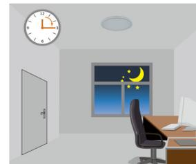
Light switches off automatically after the stand-by period elapsed
