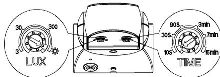
beginning. After Warm-up 30sec, the sensor can start work. If the sensor receives the induction signal, the lamp will turn on. While there is no another induction signal any more, the load should stop working within  $10\text{sec} \pm 3\text{sec}$  and the lamp would turn off.
